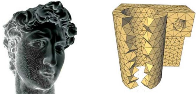
Figure 1: Typical 2D and 3D meshes: although the David's head appears smooth, its surface is made of a triangle mesh; tetrahedral meshes (such as this mechanical part, with a cutaway view) are some typical examples of irregular meshes on which faithful computations need to be performed. David's head mesh is courtesy of Marc Levoy, Stanford.
