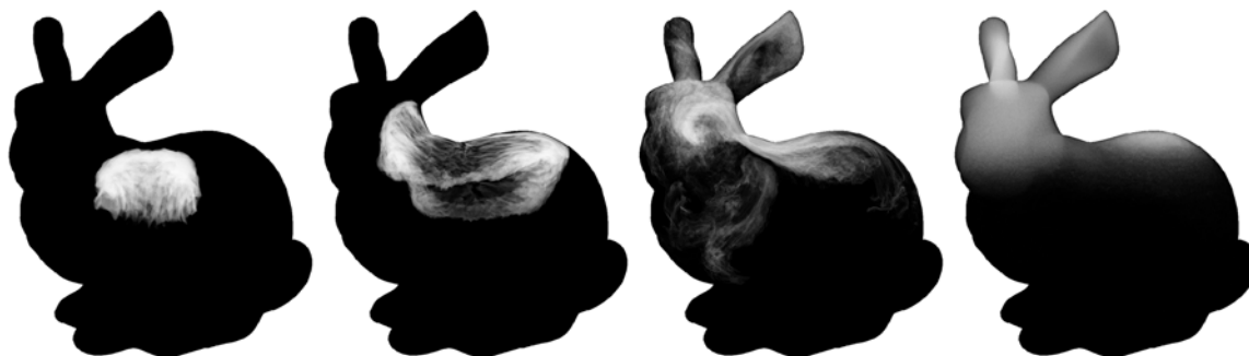
Figure 1: Discrete Fluids : we present a novel geometric integration scheme for fluids applicable to tetrahedral meshes of arbitrary domains. Aside from resolving the boundaries precisely, our approach also provides an accurate treatment of vorticity through a discrete preservation of Kelvin's circulation theorem. Here, a hot smoke cloud rises inside a bunny shaped domain of 7K vertices (32K tets—the equivalent complexity of a regular 19^3 grid), significantly reducing the computational cost for such an intricate boundary compared to regular grid-based techniques (0.47s/frame on a Pentium 4, 3GHz).
