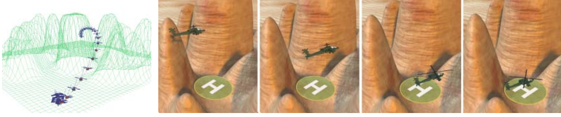
Fig. 12: Optimized trajectories of a helicopter flying through in a complex canyon (left), and automatically landing on the mark (right).
