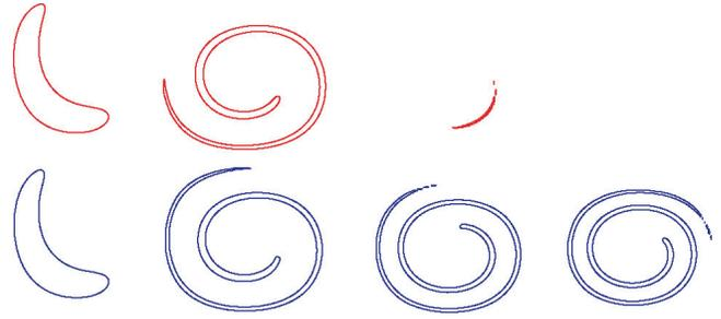
Figure 3: **2D Comparison With LSM:** Results of advecting a circle in a vortex flow via the LSM (top) and our method (bottom), both using WENO-5. Our density-based approach continues to capture the motion long after the level set has disappeared due to volume loss during advection. Grid size:  $128^2$
