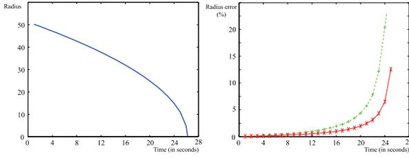
Figure 5: **Mean Curvature Flow**: (left) a mean curvature flow of a circle results in a continuous decrease of the radius; (right) when simulated in an Eulerian setup, our approach (solid line) follows the analytical value of the radius closer than the LSM (dashed line) of equivalent order (WENO-5). Grid Size:  $128^2$
