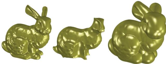
Figure 4: **Surface Offsetting:** bunny undergoes a negative and positive offset via normal flow. Notice the sharp corners properly created in the process. Grid Size:  $350^3$ .
