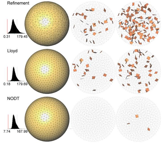
**Figure 4:** Comparing Delaunay refinement and mesh optimization. Distributions of dihedral angles are shown to the left. Slivers are shown for a dihedral angle bound of respectively 5 (middle) and 10 degrees (right). Top: Delaunay Refinement alone (resp. 35 and 136 slivers). Middle: Optimized mesh with 100 Lloyd iterations (resp. 23 and 55 slivers). Bottom: Optimized mesh with 100 NODT iterations (resp. 0 and 3 slivers).
