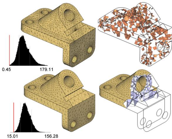
**Figure 2:** *Top:* Mesh (5,499 vertices) generated by Delaunay refinement (shape and boundary approximation criteria activated). Notice the cluster in the middle of the armhole. Right image shows tetrahedra with dihedral angles smaller than 15 degrees. *Bottom:* Mesh (3,701 vertices) generated by interleaving Delaunay refinement and optimization so as to satisfy the same criteria. Distributions of dihedral angles are shown on the left.
