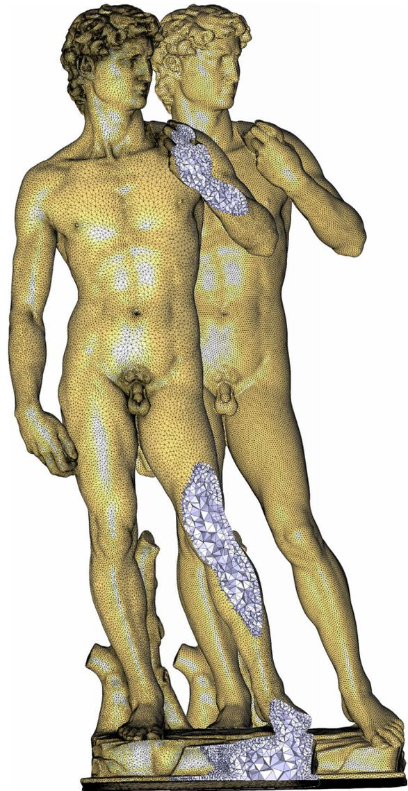
**Figure 1:** Michelangelo's David. Our mesh generation algorithm produces high quality meshes through Delaunay refinements interleaved with optimization. The input PSC has 800K triangles; (right) a uniform sizing criterion generates a 1M vertices mesh; (left) approximation error and shape criteria alone generate a smaller graded mesh (250K vertices), while guaranteeing the same mesh quality and a better local approximation error.
