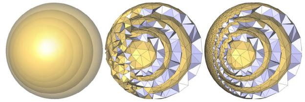
**Figure 8:** Nested spheres. Left: input PSC. Middle: mesh generated by refinement with  $l_{max} = 1$ ,  $\epsilon_{max} = 0.03$  and topology criterion not activated. Right: mesh further refined with same criteria but with topology activated.
