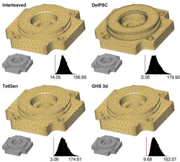
**Figure 7:** Cover rear. Top left: mesh obtained by interleaved refinement and optimization with  $l_{max} = 0.1$ ,  $\epsilon_{max} = 0.001$ ,  $\sigma^f_{max} = 1.5$ ,  $\sigma^t_{max} = 1.5$ , with topology criterion activated; 4,050 vertices. Top right: mesh generated by DelPSC, same parameters; 15,157 vertices. Bottom: meshes generated by TetGen (left, 4,189 vertices) and GHS 3D (right, 6,641 vertices), same parameters and with the boundary of our optimized mesh taken as input.
