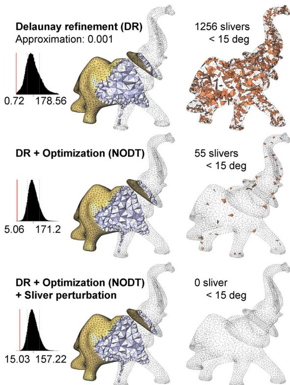
**Figure 10:** Elephant. Top: mesh generated by Delaunay refinement with  $l_{max} = 0.1$ ,  $\epsilon_{max} = 0.001$ . Distribution of dihedral angles, and sliver tetrahedra with dihedral angles lower than 15 degrees are shown. Middle: output of Delaunay refinement (i.e., top row) optimized with our technique. Bottom: optimized mesh (middle row) after sliver perturbation.
