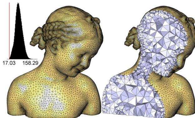
**Figure 5:** *Bimba*. Mesh generated by interleaved refinement and optimization with  $l_{max} = 0.1$ ,  $\epsilon_{max} = 0.0005$ .
