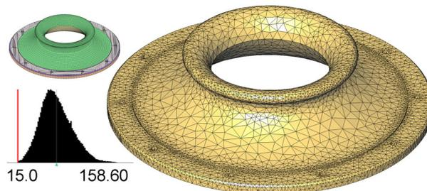
**Figure 6:** *Turbine*. Mesh generated by interleaved refinement and optimization with  $l_{max} = 0.1$ ,  $\epsilon_{max} = 0.001$ . The inset shows the input PSC with all patches segmented. The mesh has 14K vertices and 51K tetrahedra, with all dihedral angles greater than 15 degrees.
