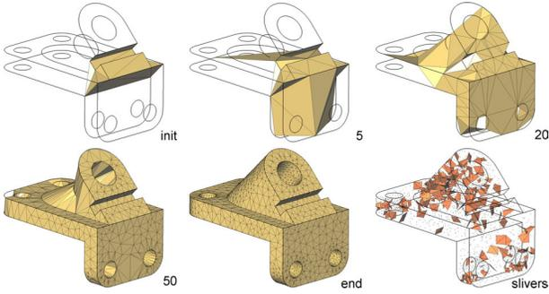
**Figure 3:** Refinement steps without optimization. The mesh initialized with feature vertices; after a few batch refinement steps (from 5 to 50); the final refined mesh with shape and approximation criteria satisfied; and its 244 slivers (tetrahedra with dihedral angle smaller than 10 degrees).
