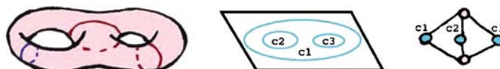
Fig. 8. A two-holed torus and its associated planar cross-section and augmented Reeb graph. To find the locally shortest nonseparating cut (shown in blue), we explore all pairs of child contours with the same component label (i.e., \{c1, c2\} , \{c1, c3\} and \{c2, c3\} ) where the minimal length nonseparating cut is associated with \{c1, c2\} .
