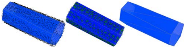
Fig. 12 Reconstruction and simplification of a cylinder. Left: 10K noisy sample points and reconstruction with 12 vertices (facet density shown). Middle: transport plan between point samples and bin centroids. Right: simplicial complex and facet density.
