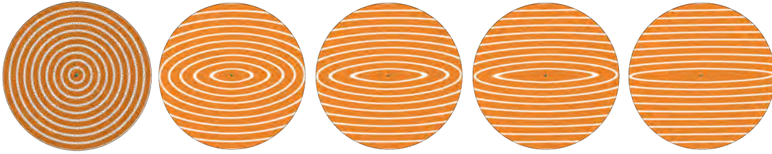
Figure 4: Our tensor-based discrete differential operators can be used to compute anisotropic geodesics. We tested our method on a disk with constant tensors of various anisotropy ratio (from left to right: 1, 0.5, 0.3, 0.2, and 0.1), with the larger magnitude along the x -axis. Notice that the iso-levels stretch to ellipses with the anisotropy as expected.
