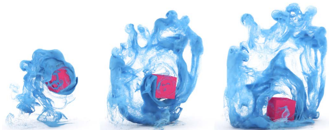
Fig. 21. Coarse-grid simulation. A falling box using one-way coupling with the surrounding fluid is computed in realtime on a coarse 50 \times 100 \times 50 grid. Due to our solver accuracy, turbulence details are still well captured.
