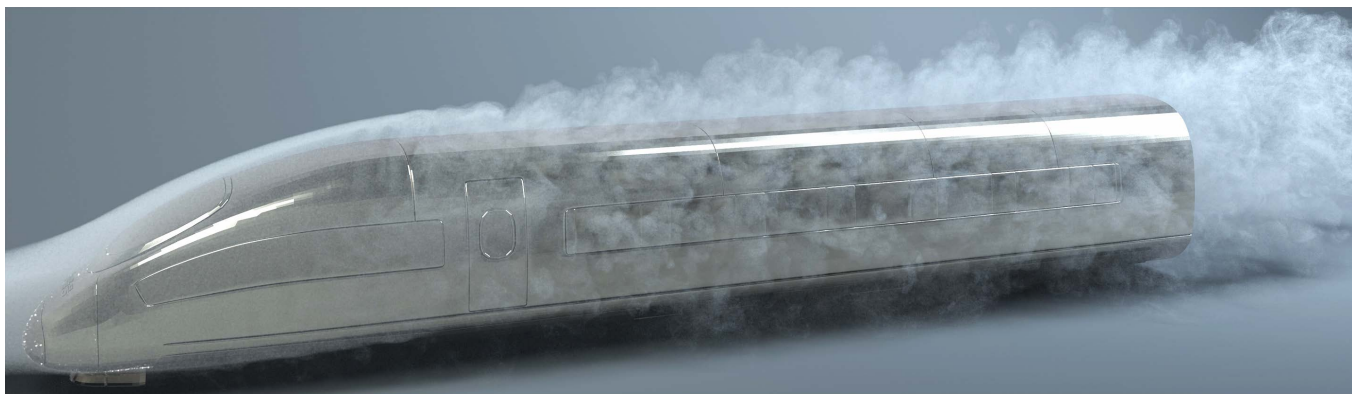
Fig. 31. Large-scale virtual wind tunnel. A static high-speed train is placed in a virtual wind tunnel (pushing air from the left); at a Reynolds number of Re=28,000 and with no-slip condition inducing boundary layer turbulence, passive white particles visualize the flow separation and ensuing vortices. This simulation was computed at a resolution of 1800 \times 400 \times 400 on a 4-GPU server, each frame (i.e., 1/50 of a second) requiring 142 seconds to simulate.
