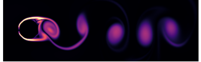
Fig. 1. Von Kármán vortex street. A vorticity plot of a simulation of a single-phase flow past a round obstacle in 2D shows the typical vortex shedding, even when a velocity-based (pressure-velocity) formulation based on distribution function g instead of f is used.
