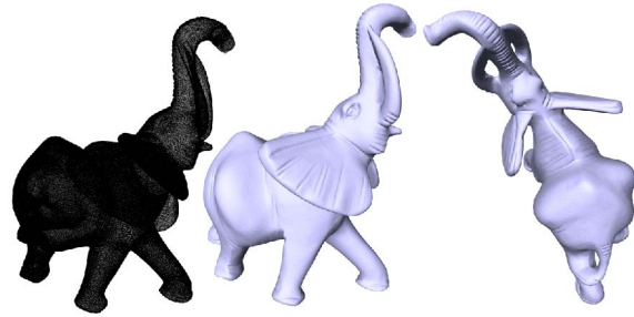
Figure 8: Stone Elephant. Pointset from a Minolta laser scanner (left) and reconstruction, seen from two angles.
