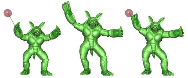
Figure 4: Length Constraint : The Armadillo's right hand is dragged while its left hand and the feet are held fixed (left). Without length constraint, the body stretches out to fit the point constraint (middle). With length constraint, no stretching occurs (right).
