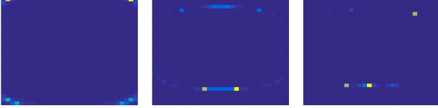
FIG. 3. Irrelevant eigenvectors. Eigenvectors of Aref's blinking vortex flow for \mu = 0.5 . Most of the eigenvectors of a Burau matrix are nearly constant (left), or only show faint parts of coherent structures (middle/right); here, eigenvector 12, 426, and 574. Compare these results with Fig. 5(bottom right) showing an eigenvector that clearly reveals dynamical structures.
