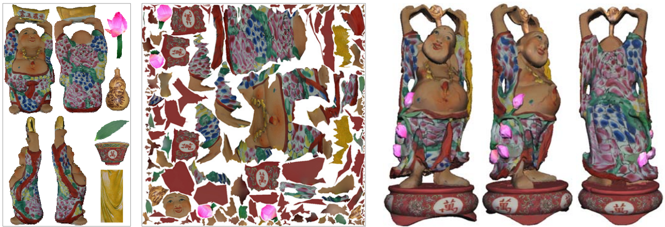
Figure 10: Texturing Buddha from textures of multiple objects. From left to right: input images, generated texture atlas and mapping results.
