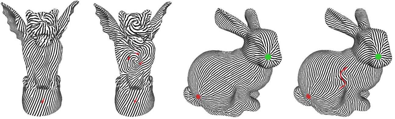
Figure 8: On the gargoyle model, a single edge constraint induces a global field; adding 3 closely spaced edge constraints creates a spiral. On the bunny model, a single source/sink pair produces the field on the left which is then reshaped with a curve constraint drawn on the body.
